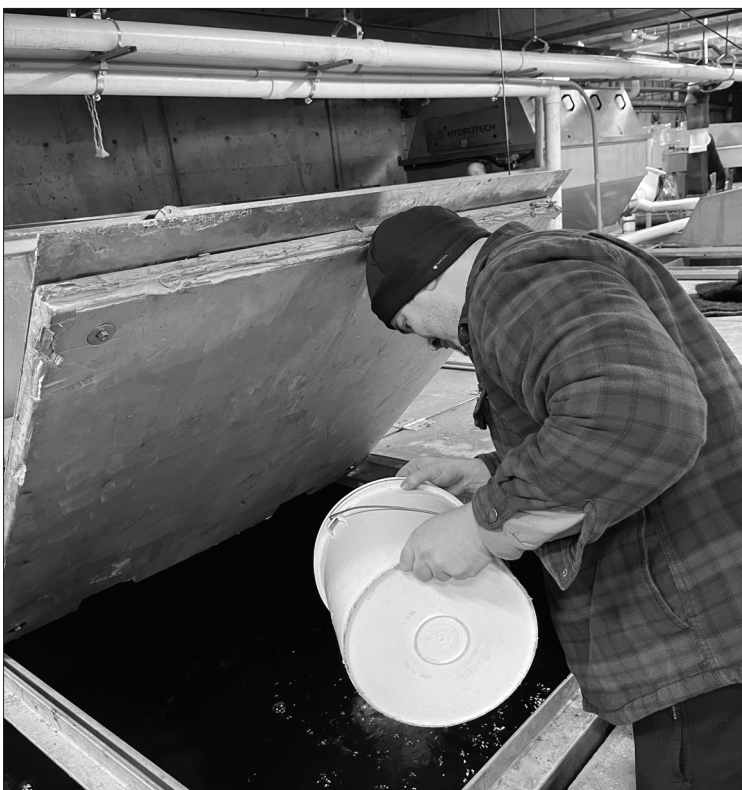
Sodium Bicarbonate being added to the water system
